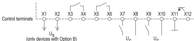
The input resistance of the control inputs is 80kOhms. To control them, it is necessary to use switching contacts enabling reliable switching of the lower control currents (e.g., AgNi+Au)!
